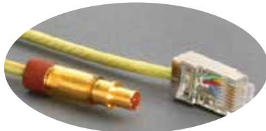
Quadrax Pin with 8P8C "RJ45" Jack
